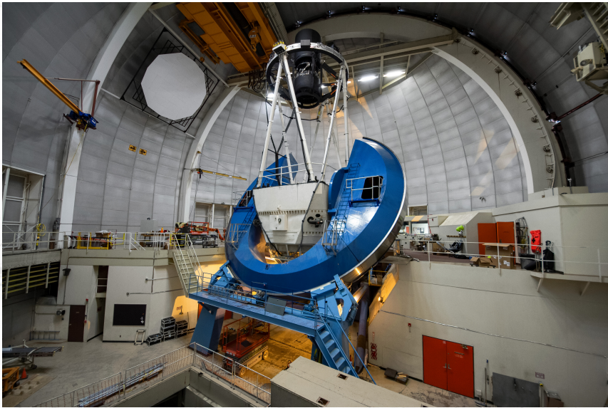
DESI is mounted on Kitt Peak National Observatory's Nicholas U. Mayall 4-meter telescope.
