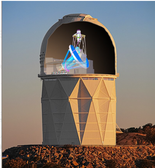
The Dark Energy Spectroscopic Instrument (DESI). DESI installed on the Nicholas U. Mayall 4-meter Telescope at Kitt Peak National Observatory.
