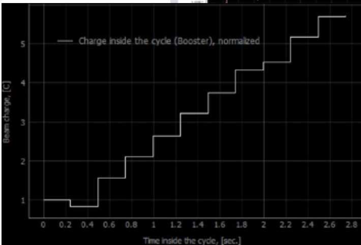
Sixfold increase in beam intensity of Xe ions in Booster with 10x injection
