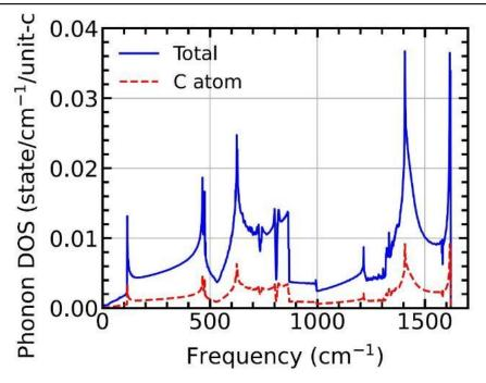
The PhDOS characterizes graphite vibrations. The total PhDOS (solid blue) is reported per primitive unit cell, and the partial density of states (PDOS, dashed red) is the site-averaged contribution per carbon atom. With this normalization, summing the per-atom PDOS over the four atoms in the cell gives the total. Low-frequency peaks arise from interlayer shear and breathing motions, whereas highfrequency peaks correspond to in-plane optical modes near 1580 cm<sup>-1</sup>.
