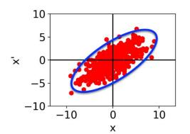
Emittance ( $\epsilon$ ) is the phase space volume occupied by the beam in coordinate-momentum space (x, x').  $\epsilon_n = \gamma \beta \epsilon \epsilon_n$  is invariant of motion
