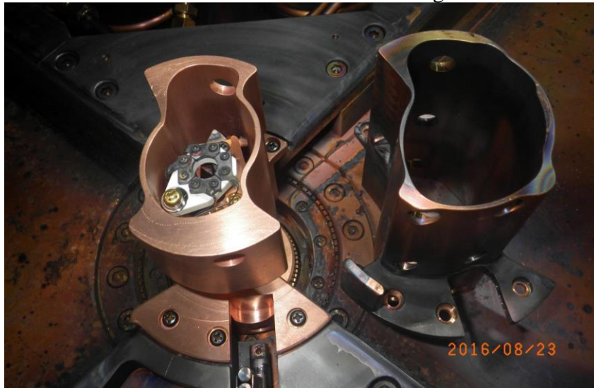
Figure 31: Photograph of the RF shields around the inflector.
