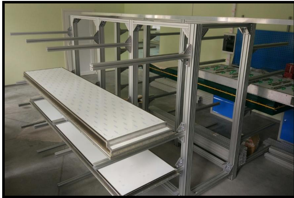
1 stand = 6 modules = 60 detectors (120 preamps + 40 TDC)
