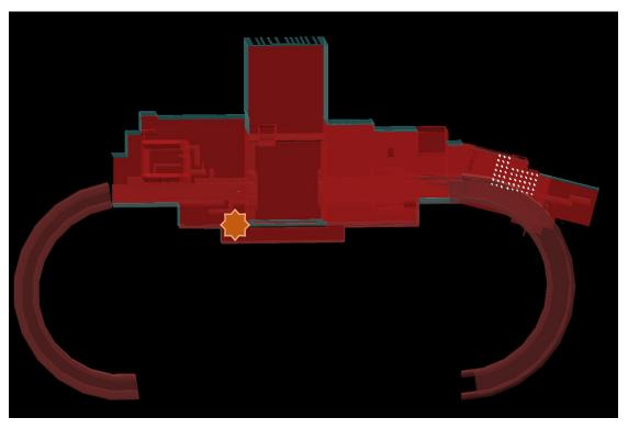
NICA model in Geant4, white dots indicates detectors in the Temporary control room.
