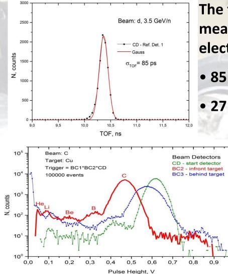
Study of beam and pulse height resolution of detectors.
