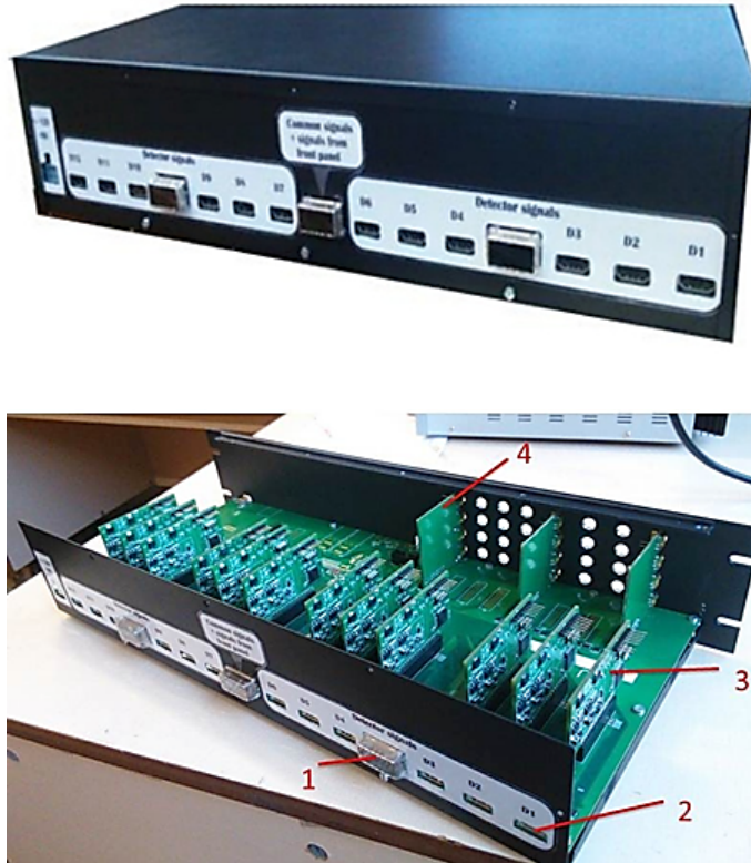
A photo of T0U module: 1 - the output Molex connector; 2 - the input HDMI connector; 3 - the power supply board; 4 - the IOB output connectors of trigger signals generated by T0U.
