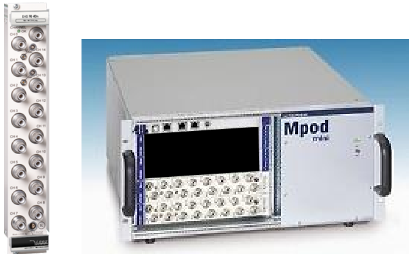
A view of the 16- channel HV module and HV crate
