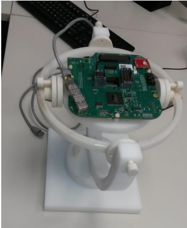
Gyro-gimbal for AHRS calibration
