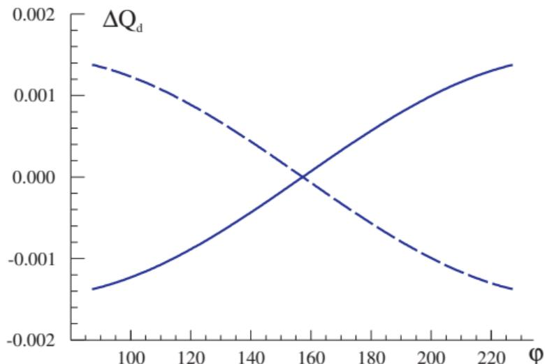
Dependences of  $\Delta Q_d$  on  $\varphi$  with negative (dashed line) and short-time positive (solid line) feedback modes
