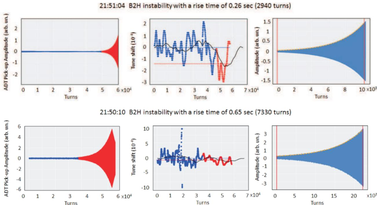
The active feedback system can be used as a source of controlled an arbitrary complex tune shift.
