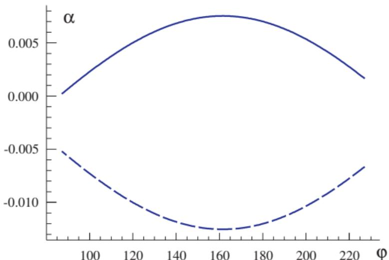
Dependences of increment (solid line) and decrement (dashed line) on Hilbert filter parameter  $\varphi$  at fixed gain  $g = 0.02$
