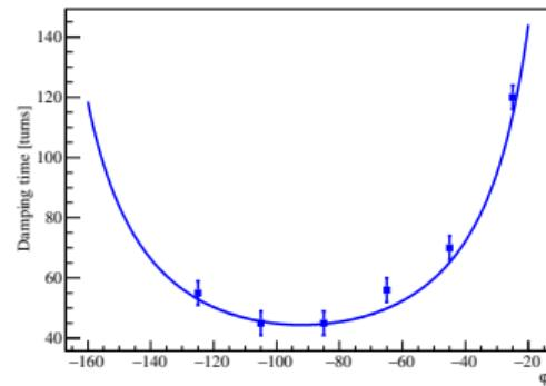
Fractional tunes  $\{Q\}$  (left) and damping times  $\tau_d/T_0$  (right) in dependence on the Hilbert filter parameter  $\varphi$  at  $Q_0 = 64.278$  and  $\hat{q} = 2$  (Experimental data from: Höfle W. et al. LHC Transverse Damper Observations versus Expectations. CERN-ATS-2011-017. Pp. 107–114.)
