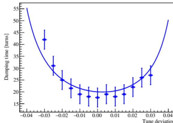
Tune shifts  $\Delta Q_d$  (left) and damping times  $\tau_d/T_0$  (right) in dependence of the tune deviations  $\Delta Q_0$  from  $Q_0 = 59.295$  at  $\hat{q} = 0$  (Experimental data from: Komppula J. et al. MD4036: New ADT signal processing for large tune acceptance. CERN-ATS-NOTE-2019-0008).
