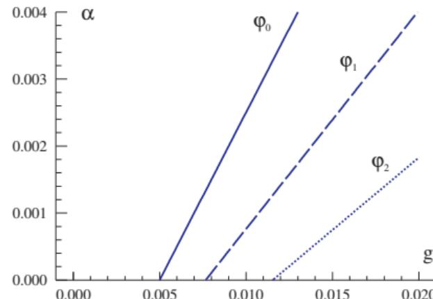
Dependence of increment  $\alpha$  on gain  $g$ :  $\varphi_0 = \varphi_{\text{opt}}$  (solid),
