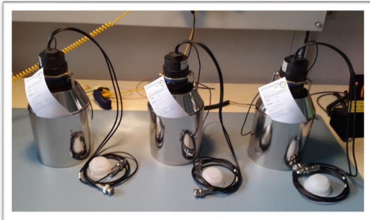
PMTs with Mu-Shield (3x ETEL 9821, 3inch)
