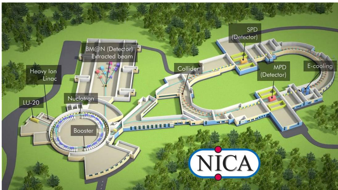
Figure 1: Layout of the NICA collider with SPD at the south collision point.
