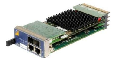
**For several MTCA modules one main MCH concentrates data from slave MCHs to generate the final muon trigger**
