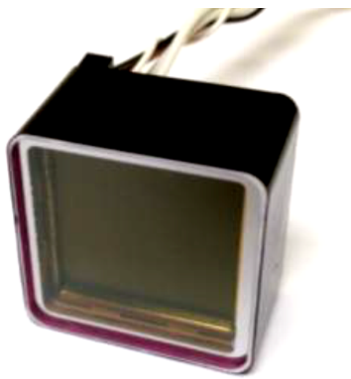
MCP-PMT XPM85112/A1-Q400 (Photonis) Photocathode: 25 × 25 mm 2
