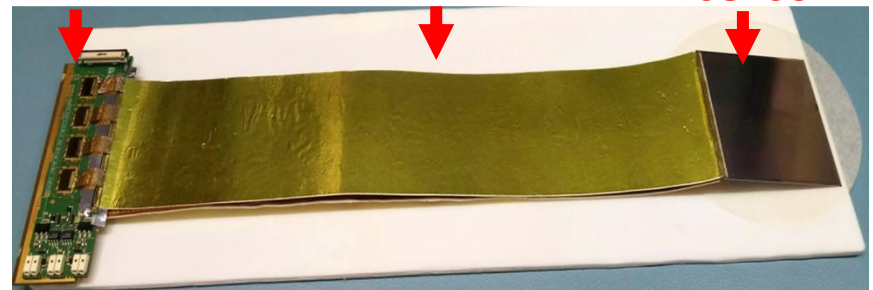
First assembled module with 62x62 mm 2 sensor
