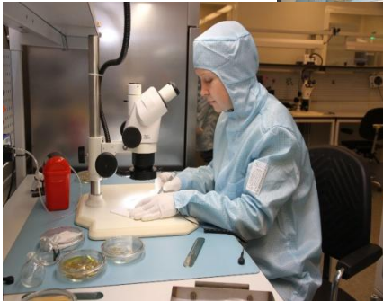
Assembling of the mockups of BM@N STS modules
