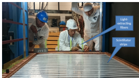
Mounting of the 1 st section of the DANSS calorimeter (KNPP; 19.08.2015)
