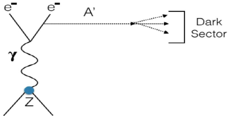
*NA64 is a fixed target experiment combining the active beam dump technique with missing energy measurement searching for invisible decays of massive  $A'$  produced in the reaction  $eZ \rightarrow eZA'$  of electrons scattering off a nuclei ( $A, Z$ ), with a mixing strength  $10^{-5} < \epsilon < 10^{-3}$  and masses  $M_{A'} < 100$  MeV.*
