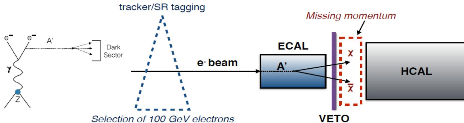
For NA64 a beam of **100 GeV electrons** will be dumped against an ECAL, a sandwich of lead and scintillators ( $34 X_0$ ), to produce massive  $A'$  through scattering with the heavy nuclei.
