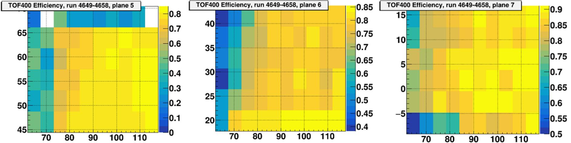
Examples of the efficiency distributions for the ToF – 400 planes (right arm, CSC is not installed)
