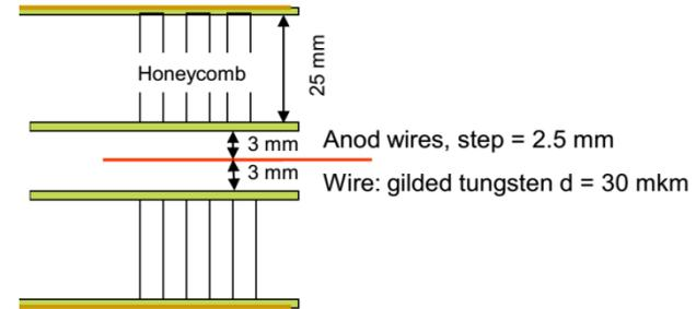
Two cathode planes with strips inclined at 0° and 15°
