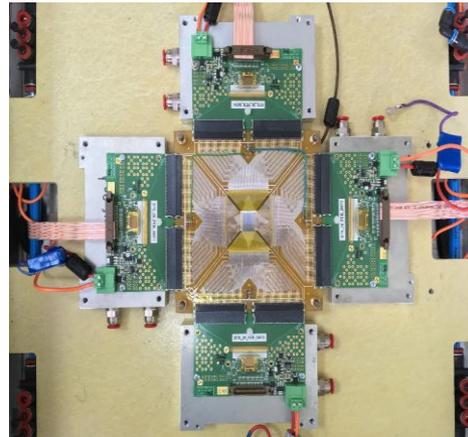
STS1,2 – Test stations with double-sided microstrip silicon sensors
