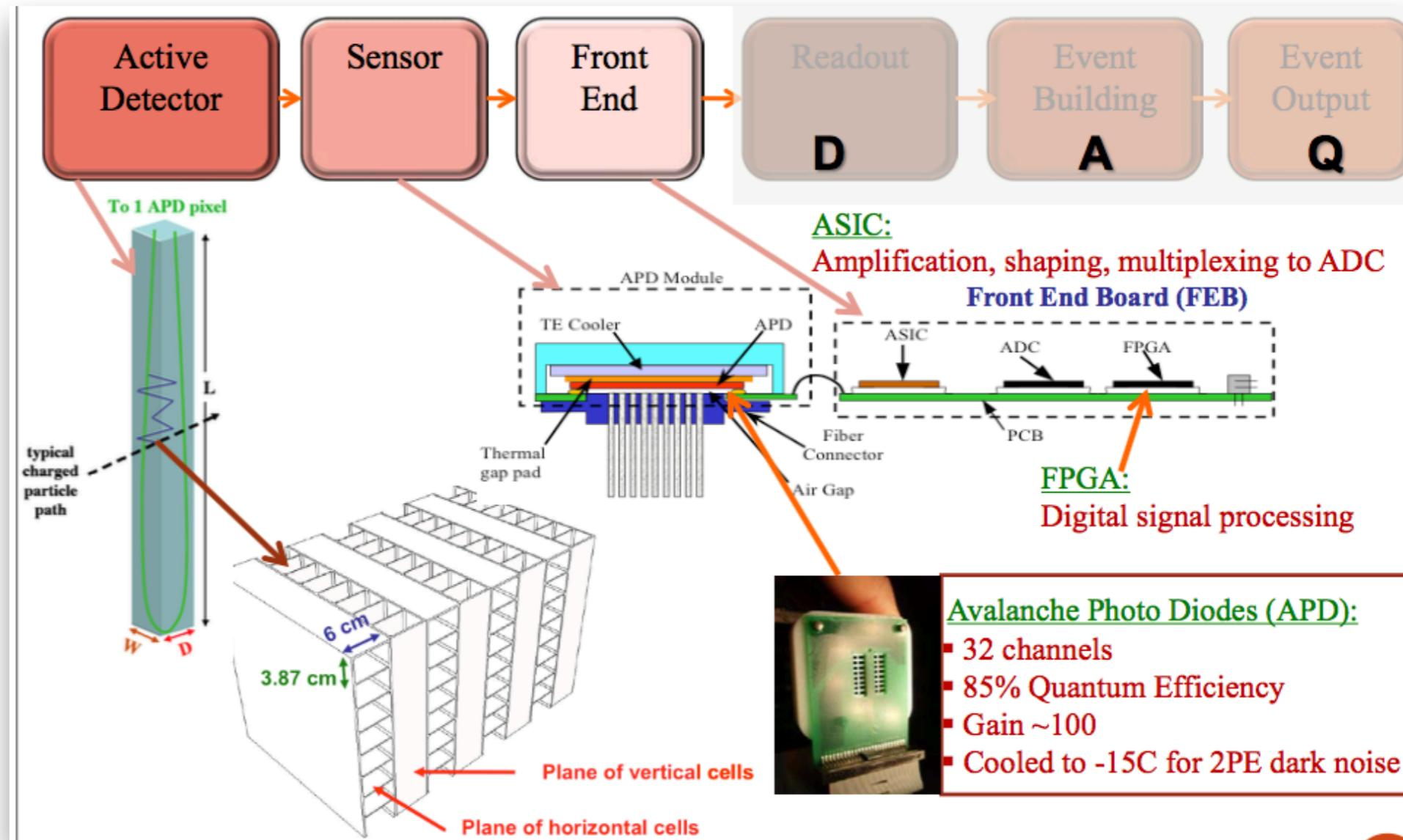
SIGNAL SHAPING: Scintillator -> Fiber -> APD -> FEB
