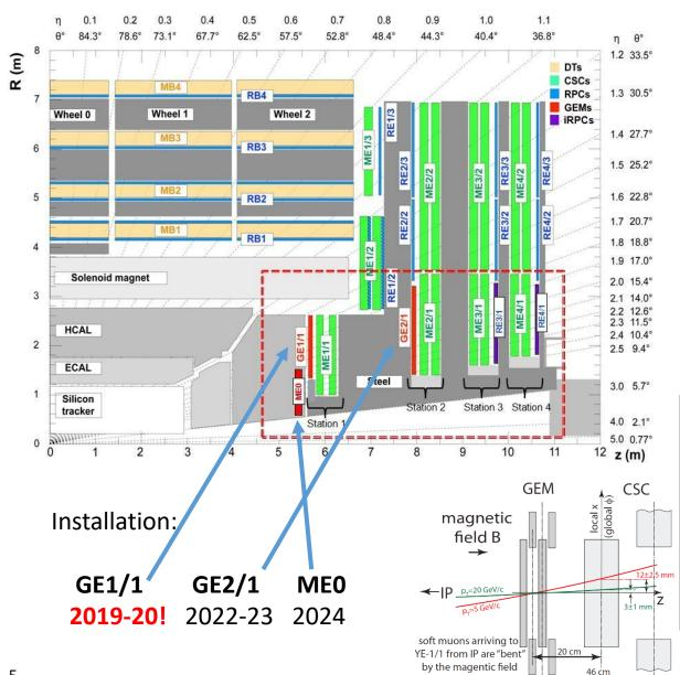
Three new muon stations using Gas Electron Multiplier (GEM) technology
