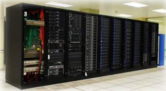
Large Offline data center at CC-IHEP ~4000 CPU cores and 4PB disk storage, 20PB tape storage for simulation, reconstruction, analysis, data storage and archive
