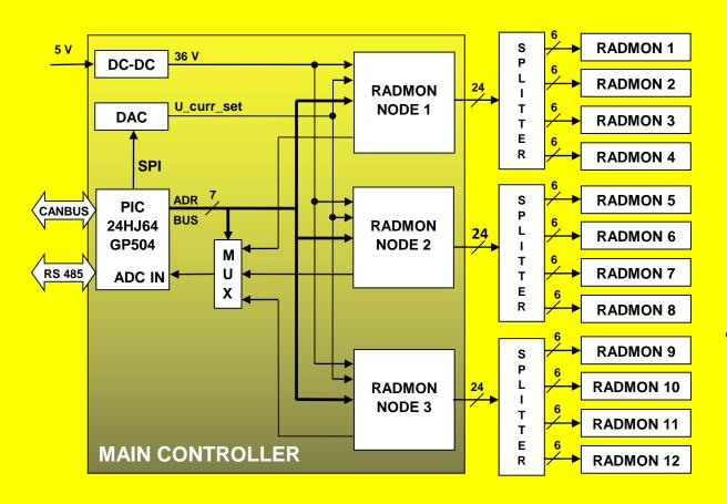
The system consists of a **Main Controller** and a basic radiation sensor unit, called **RADMON. Up-to** 12 RADMONs can be connected to the main controller.
