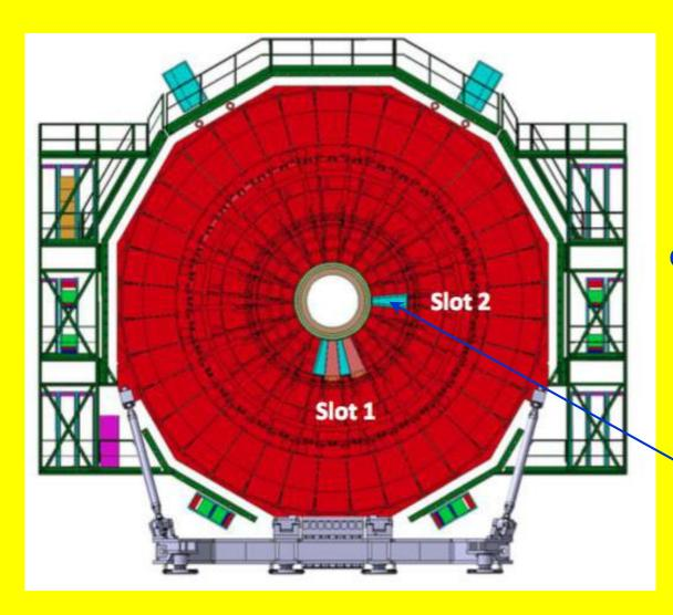
Three GEM detector prototypes were installed in March 2017 insight two slots of the GE1/1 station in inner endcap of CMS for a slice test
