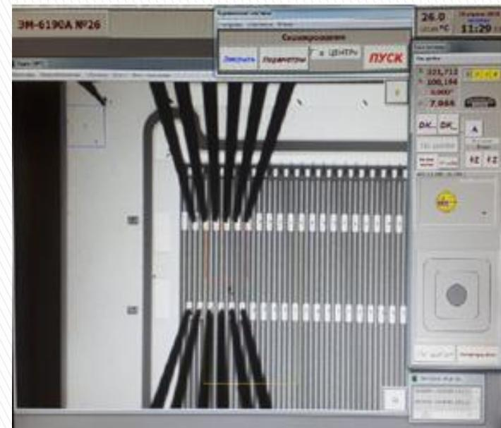
Fragment of alignment of the contact pads of the sensor with probes
