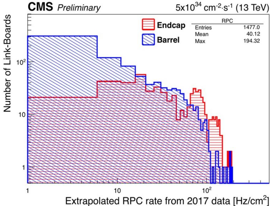
*Linear dependence on the instantaneous luminosity has been used to extrapolate the RPC rates to the HL-LHC conditions and luminosity of  $5 \times 10^{34} \text{ cm}^{-2} \cdot \text{s}^{-1}$ .
