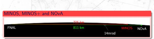
Cross section of the earth showing Fermilab, MINOS and NOvA, to scale. The red line is the central axis of the NuMI beam.
