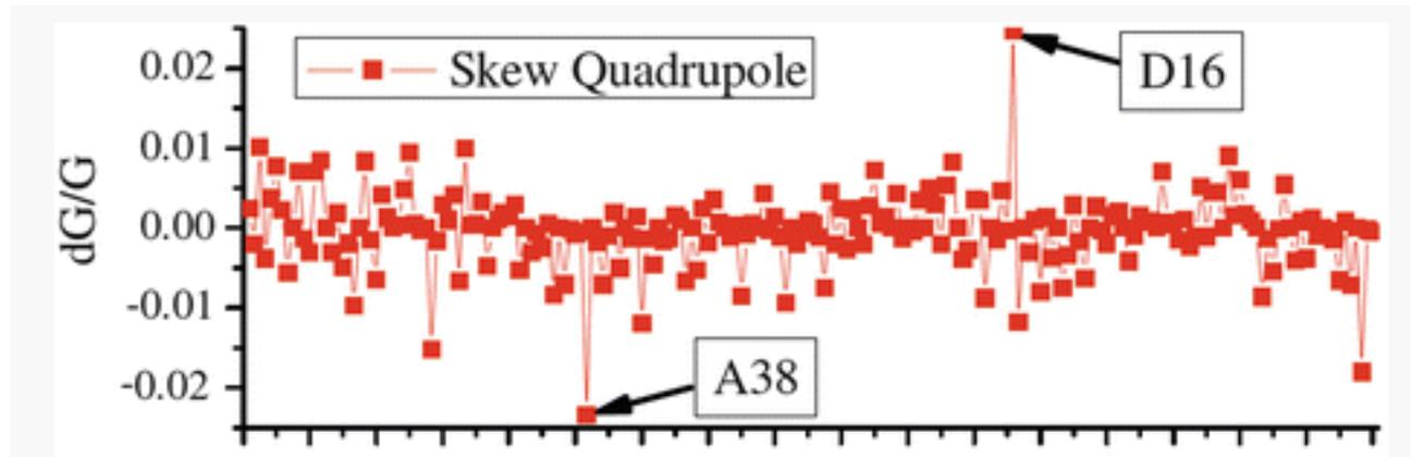
It was found that the quadrupoles at A38 and D16 were erroneously assembled with a large roll angle undetectable by alignment measurements outside of the magnet.
