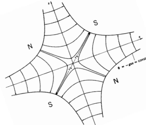
For a perfectly aligned pure skew quadrupole (a normal quadrupole rotated by 45 degrees around the longitudinal axis) the equations of motion are simply
