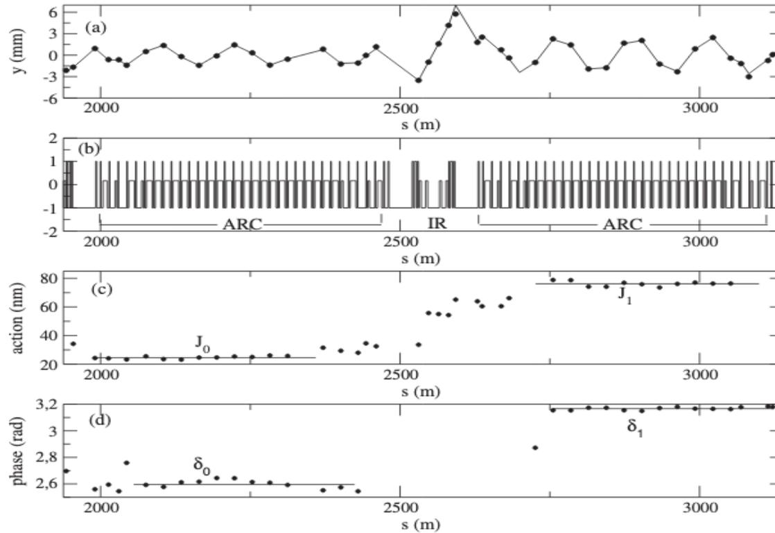
FIG. 8. (a) One of the first difference orbits obtained from beam in RHIC in the year 2000. Each dot represents a BPM measurement. (b) Lattice representation of RHIC. (c) Action plot obtained by applying Eq. (13) to all pairs of adjacent BPM measurements in the ring. (d) Phase plot obtained by applying Eq. (14) to all pairs of adjacent BPM measurements in the ring.
