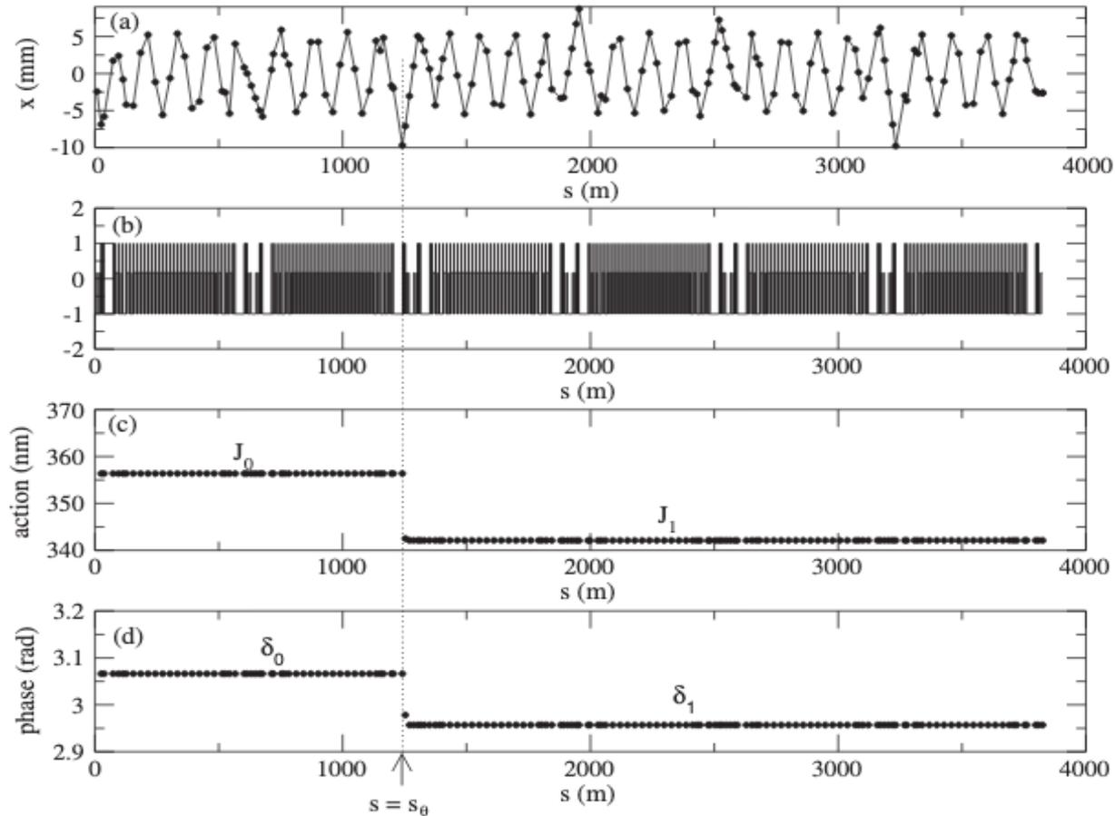
FIG. 1. (a) Simulation of a RHIC first turn trajectory with every dot representing a BPM measurement, in the presence of a magnetic kick with strength  $\theta_z$  at  $s_\theta = 1241$  m. (b) RHIC optics with short bars representing dipoles and long bars representing quadrupoles. (c) Action analysis of the simulated first turn trajectory. (d) Phase analysis of the same trajectory.
