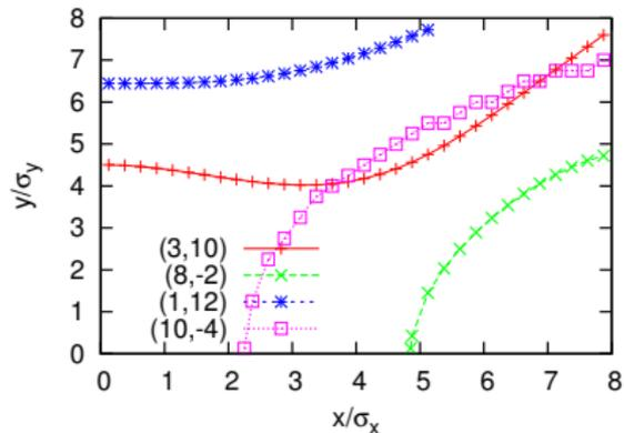
Figure: Tune spread area and resonance in the amplitude space for a hadron collider, SPPC ( $\times$ -crossing), long range collisions are included.
