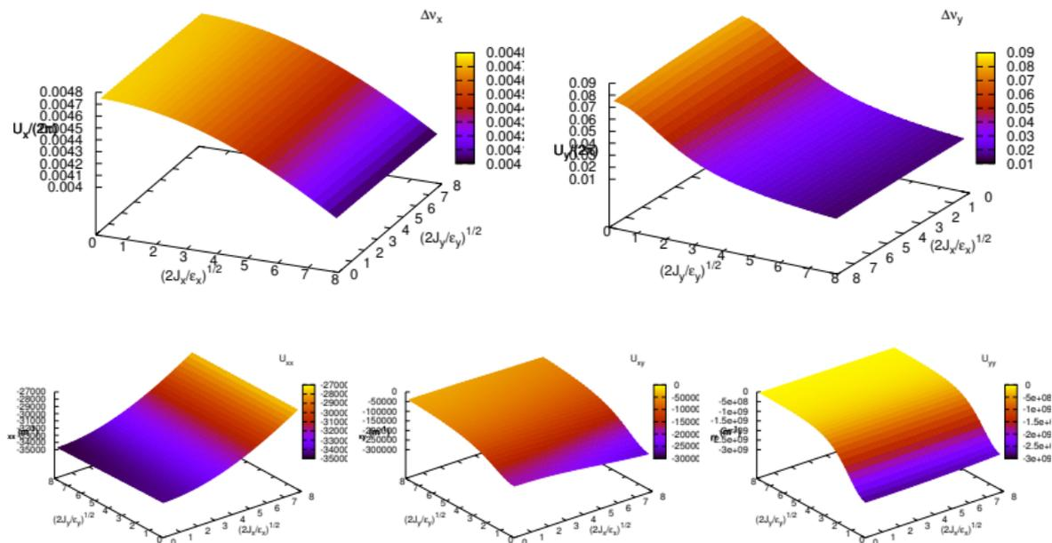
Figure: Tune spread and slope in SuperKEKB (detuned  $\beta_y = 3$  mm).
