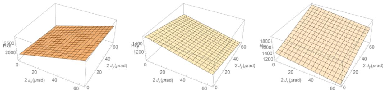
Figure: Tune slope due to lattice nonlinear magnets in J-PARC MR. (left)  $\partial^2 H / \partial J_x^2$ , (center)  $\partial^2 H / \partial J_x \partial J_y$ , (right)  $\partial^2 H / \partial J_y^2$ .
