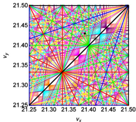
Figure: .Tune diagram near  $(\nu_x, \nu_y) = (21.39, 21.43)$
