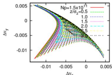
Figure: Tune spread for finite synchrotron amplitudes.
