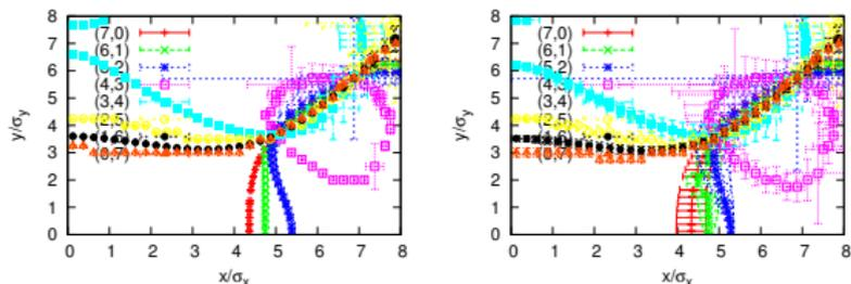
Figure: Resonance width in the transverse amplitude space for zero and finite synchrotron amplitude.
