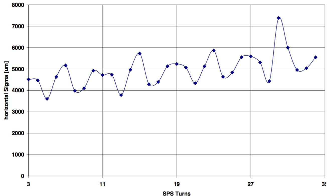
**Uncorrected measured horizontal beam size versus number of turns in the SPS. The oscillation indicates mismatch, the positive slope blow-up is due to the foil**
