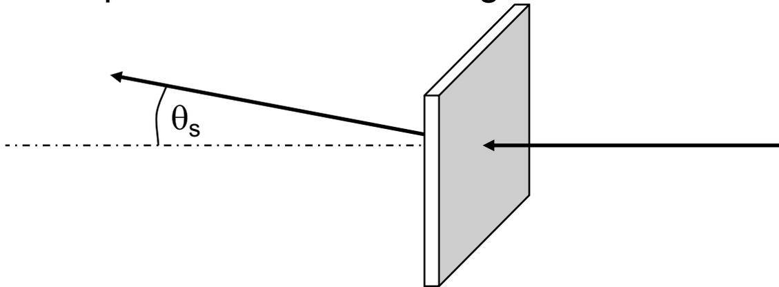
$$\text{rms angle increase: } \sqrt{\langle \theta_s^2 \rangle} [\text{mrad}] = \frac{14.1}{\beta_c p [\text{MeV} / c]} Z_{inc} \sqrt{\frac{L}{L_{rad}}} \left( 1 + 0.11 \cdot \log_{10} \frac{L}{L_{rad}} \right)$$
