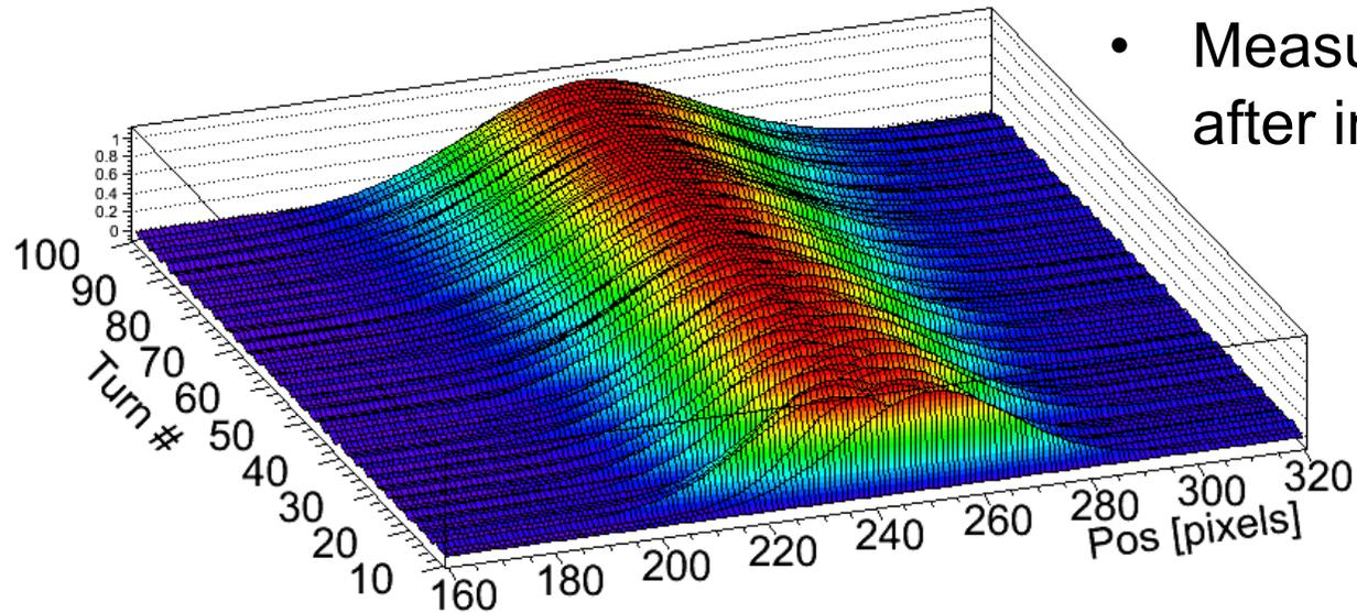
**Profiles at matching monitor after injection with steering error.**
