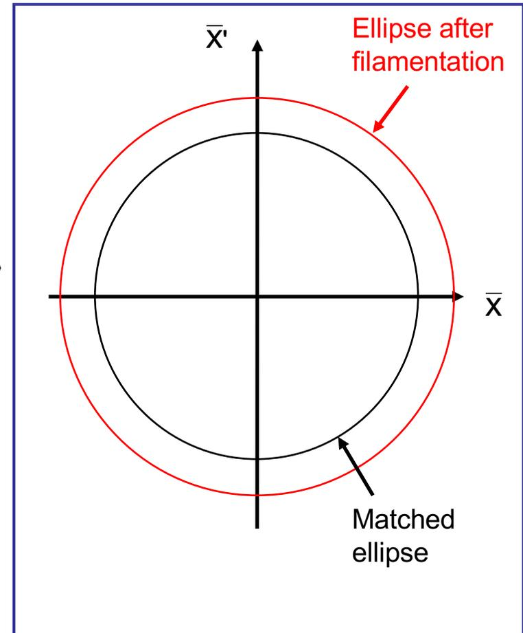
Need to keep  $\beta$  small to minimise blow-up (small  $\beta$  means large spread in angles in beam distribution, so additional angle has small effect on distn.)
