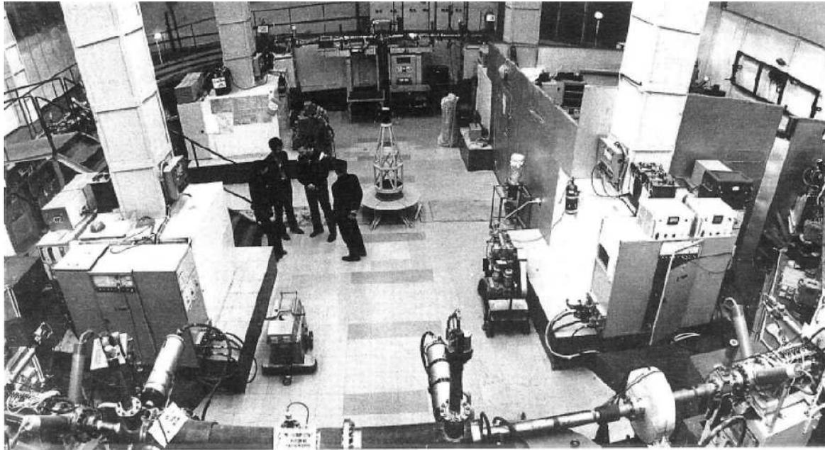
NAP-M is the first storage ring for investigation of electron cooling of ions. The injector is electrostatic accelerator with use Van de Graaff generator at 1.5 MeV. The range of energy of protons is 1.5 – 90 MeV, the proton current is up to 300 mA. The electron cooler was named EPOCHA ("Electron Beam to Cool Antiprotons") and had parameters: energy – 50 keV, electron current – up to 1 A.
