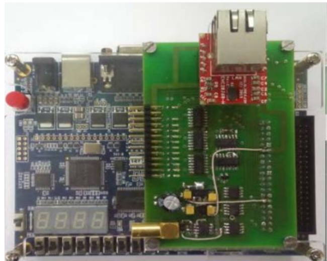
Control block for PMT scanning station
