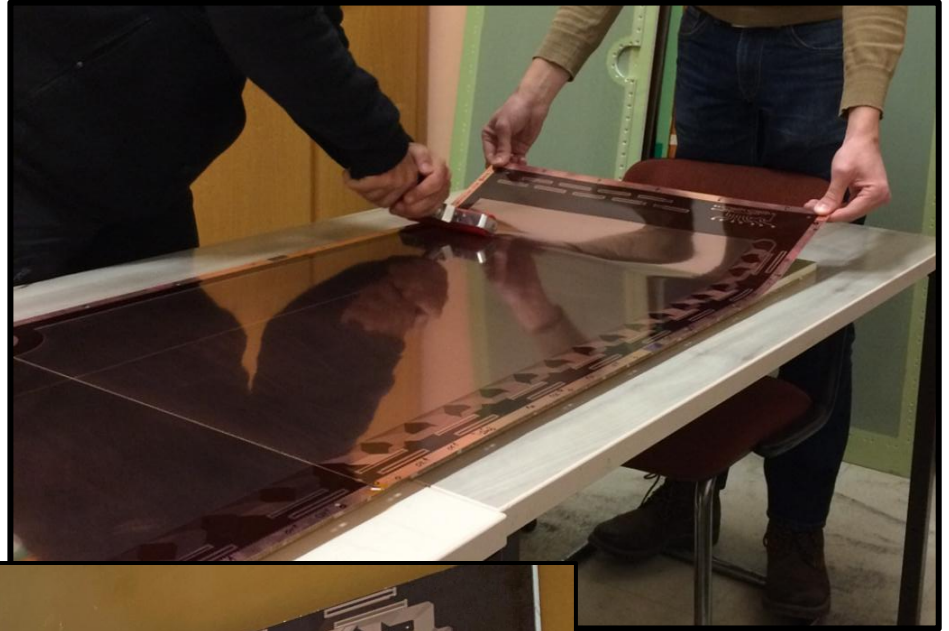
Gluing of the readout boards on the honeycomb support plate
