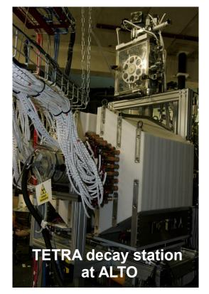
ε(1n) ~50% (measured with <sup>252</sup>Cf) ε(gamma)~1% (1MeV) ε(beta) ~ 50%
