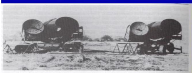
Figure 10.1 The first stellar intensity interferometer; the pilot model of the stellar intensity interferometer at Jodrell Bank in 1955. Two Army searchlights were used to make the first measurement of the angular diameter of a main sequence star (Sirius).
