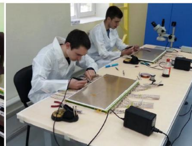
Cables and connectors soldering
