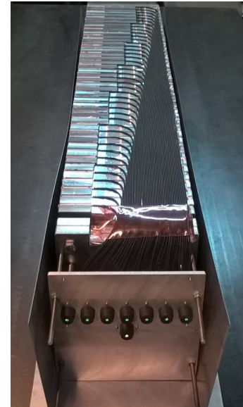
Optical connectors are polished.
