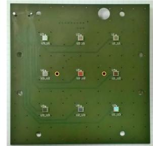
PCB is combined with the scintillator. The scintillator is divided into 9 cells.
