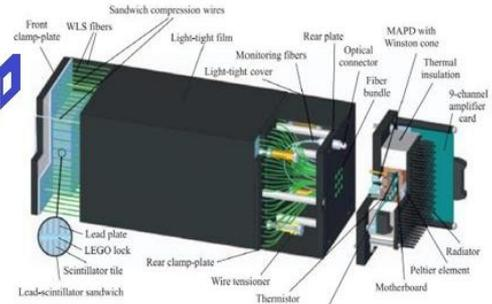
Design of the Shashlyk type calorimeter module
