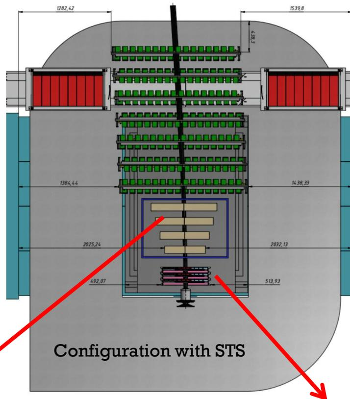
Forward Si will be removed after integration of STS full configuration into BM@N setup (2022 year, high beam intensity - few  $10^6$  Hz)
