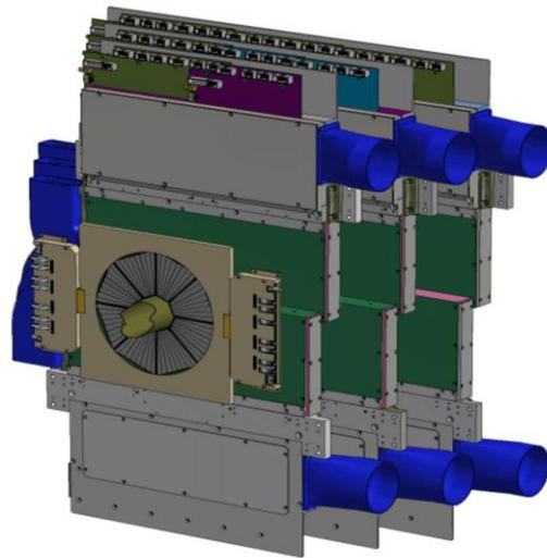
Design of the Si-planes on the BM@N beam-channel
