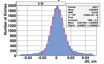
Si-3 detector residual vs GEM+Si track  $\sim 86 \mu\text{m}$
