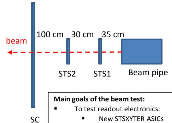
STS1,2 – Test stations with double-sided microstrip silicon sensors
