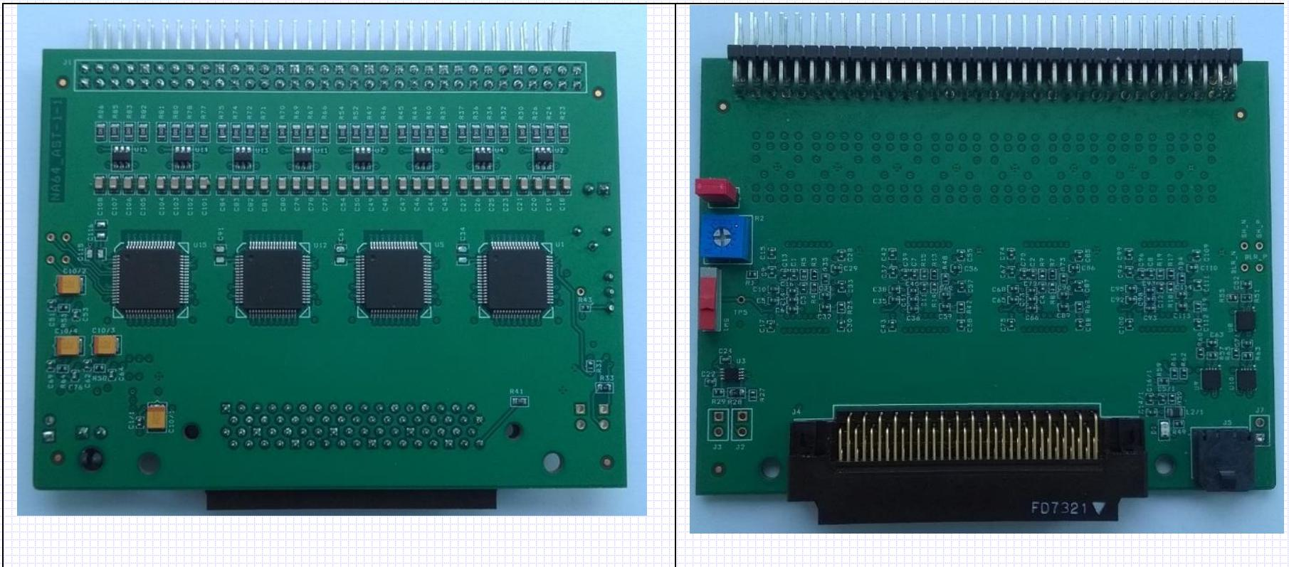
Fig. 5 Front-end electronics PCB for straw detectors
