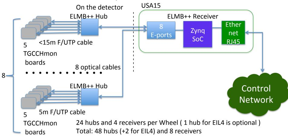
Cables: 244 15 m F/UTP cables and 8 ??? m optical cables
