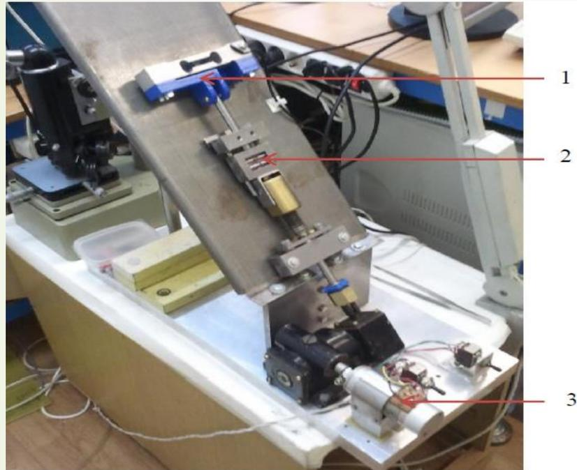
Test bench for checking of seam breaking force:
