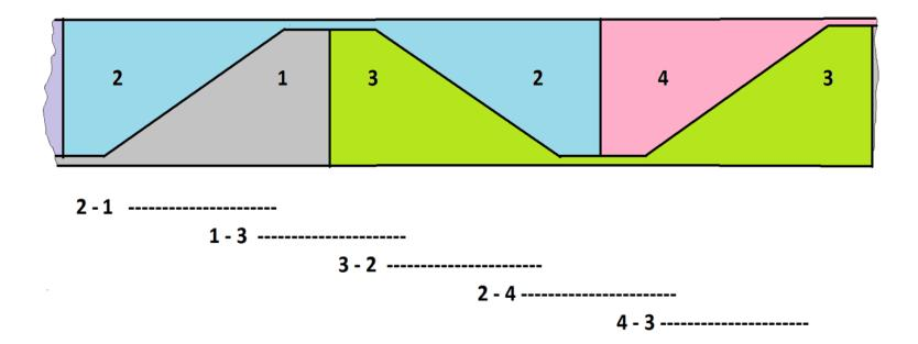
A hit is counted if the signals in two neighboring zones are above the threshold
