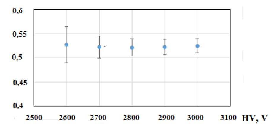
Charge ratio vs straw high voltage for a fixed Z
