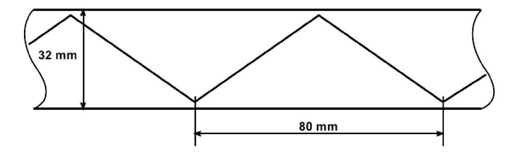
Unfolded cathode surface electrically separated into two zigzag stripes
