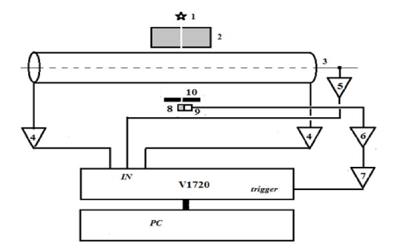
The test measurement set-up:  $1 - {}^{90}$ Sr, 2 - lead collimator ( $\emptyset$  2 mm), 3 - anode, 4 - cathode amplifiers, 5 - anode amplifier, 6 - SiPM amplifier, 7 - discriminator, 8 - scintillator counter ( $2x2x5 \text{ mm}^3$ ), 9 - SiPM, 10 - slit collimator ( $1x5 \text{ mm}^2$ ).
