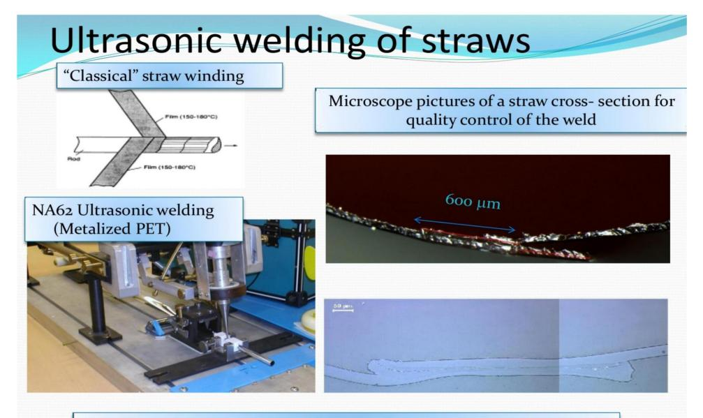
Delicate tuning of production parameters for welding
