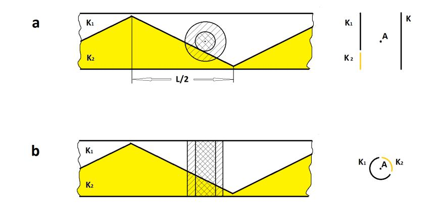
a. Planar drift cell with a periodical pattern on the cathode.b. Unrolled straw tube cathode surface with a double-wedge periodical pattern
