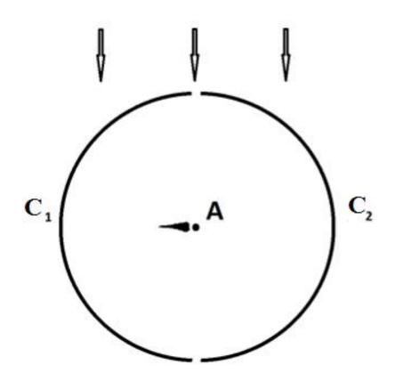
A scheme of test measurement for a straw detector with a cathode cut along the cylinder generatrix into two zones  $C_1$  and  $C_2$
