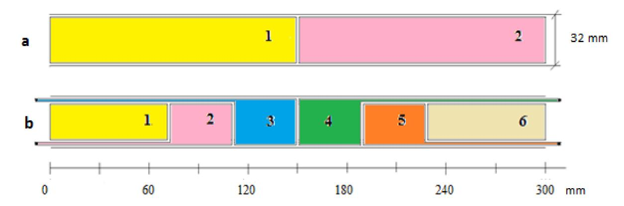
Unfolded tape for making segmented cathodes: a) 2 segments; b) 6 segments
