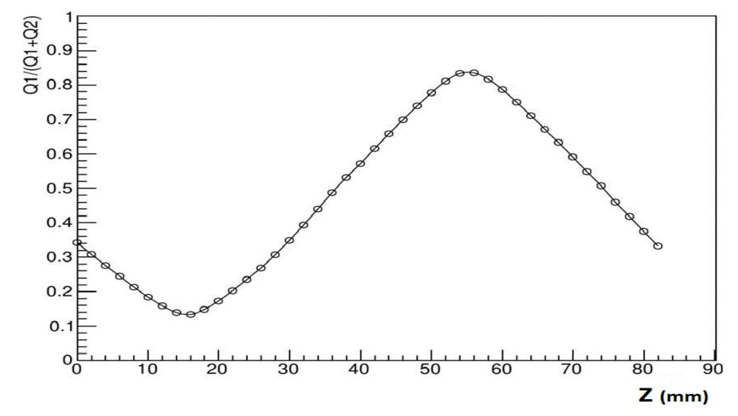
The ratio of the one strip induced charge Q1 to the total induced charge Q1+Q2 as a function of radioactive source position along the straw
