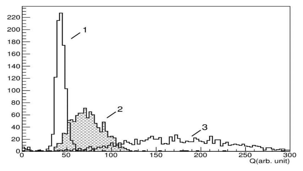
Cathode amplitude spectra for different voltages: 2650V (1), 2725V (2), 2800V (3)
