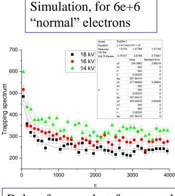
Delta of energy lost for trapped electrons before finally escaping to Spectrometer
