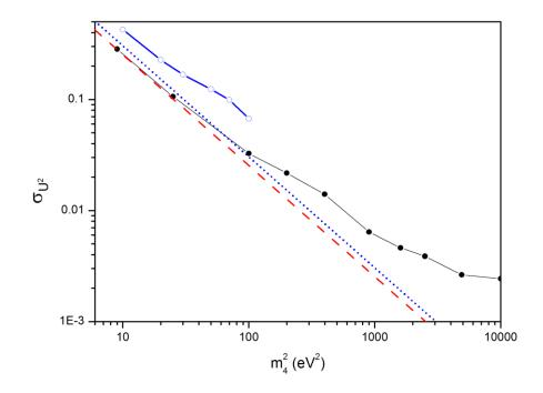
Comparison of errors for heavy eutrino mass obtained by the analysis, black symbols connected by solid lines, and approximate estimation  $\sigma(U_{e4}^2) = 2.53/m_{\nu}^2$  based on the result for the electron antineutrino mass V. N. Aseev et. al., Phys. Rev. D84, 112003 (2011), red dashed line.
