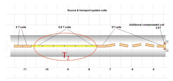
Trapped electrons can run back and forth up to thousand times passing few kilometers
