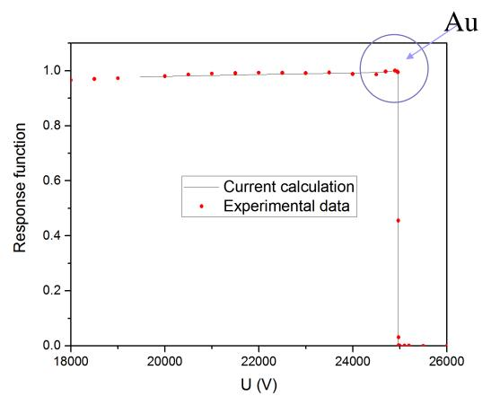
Count rate for 25 keV electrons vs spectrometer retarding potential
