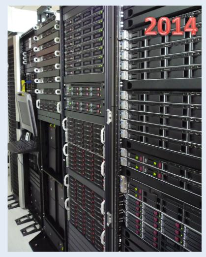
CPU: ~ 800 Cores 2.8-3.1 GHz (DELL, HP) Disk: ~ 300 TB (DELL, HP, Supermicro) GPU: nVidia (C1060, M2050, K20m)
