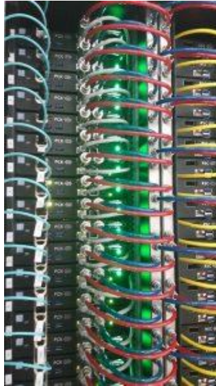
Fig.11. Supercomputer computing nodes with liquid cooling.
