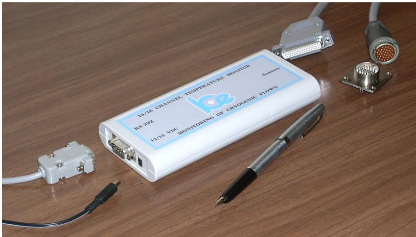
15-channel temperature monitors: upper – ISA bus, lower – RS232 (remote)
