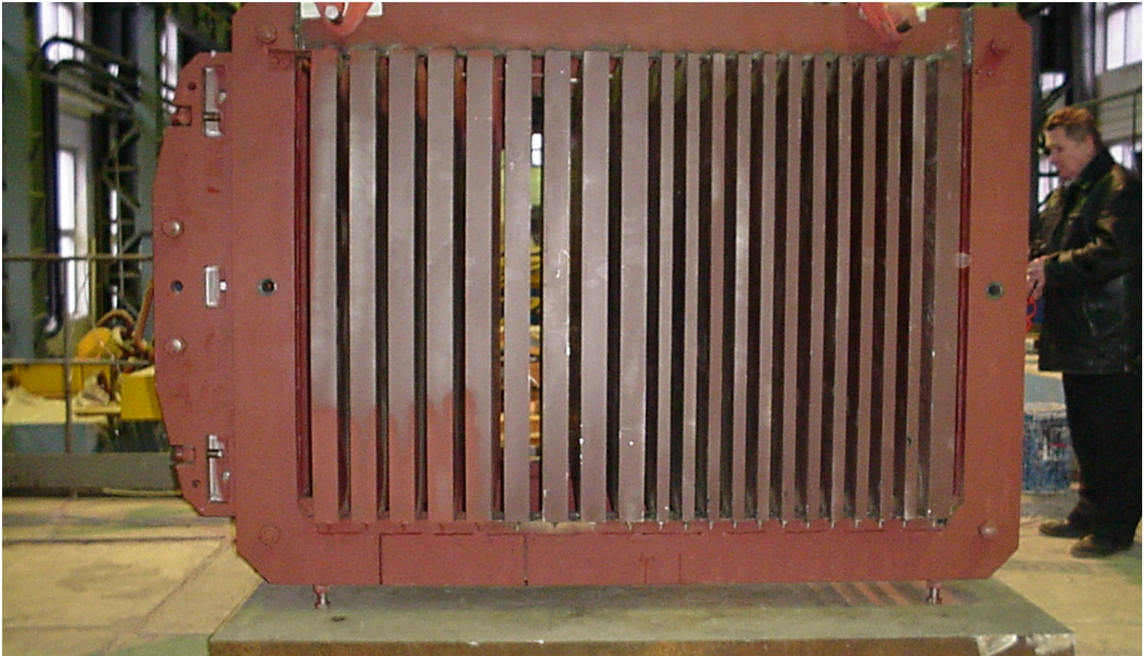
The absorber structure in horizontal position
