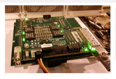
The readout electronics: FPGA based 64 channel ADC64 board, 62.5MS/s (AFI Electronics, JINR, Dubna).
