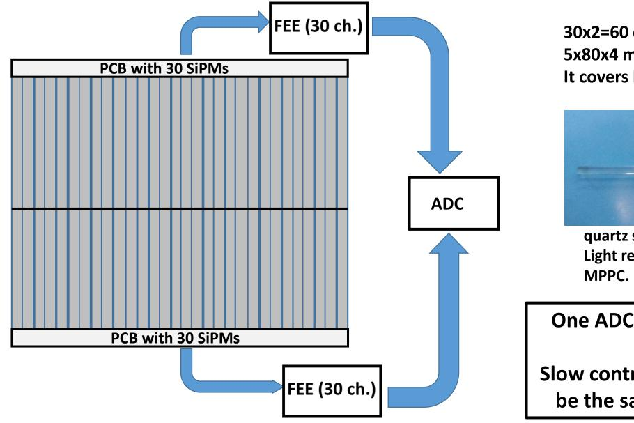
30x2=60 quartz strips; 5x80x4 mm<sup>3</sup>; It covers beam hole 15x15 cm<sup>2</sup>.
