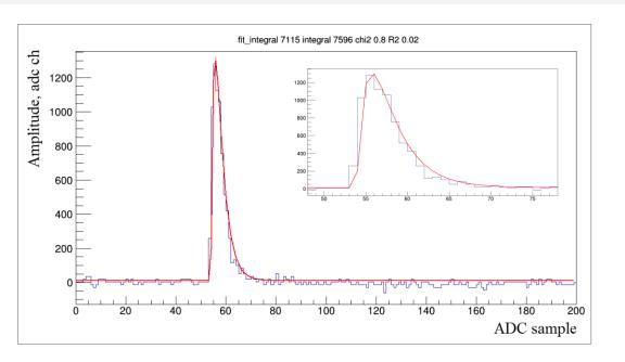
Minimum 20 ADC samples are needed to digitize the signal.
