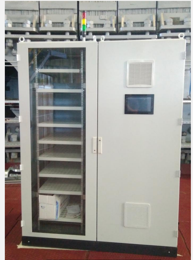
Control rack of vacuum system
