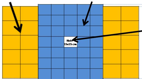
dE/dx scintillator to resolve central / peripheral interactions
