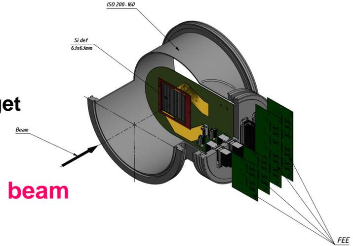
Barrel detector around target
